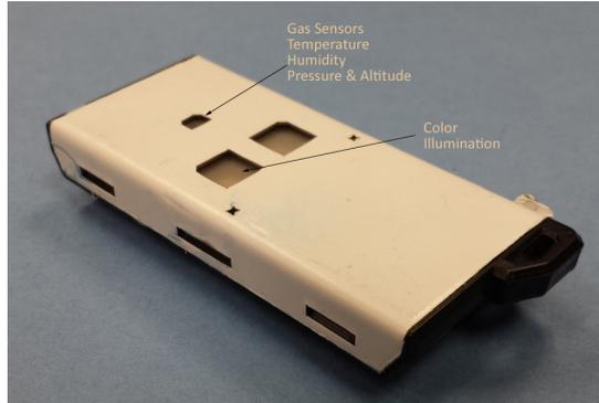
**Fig. 3.** Sensordrone device with different sensors (ambient temperature, precision gas, humidity and altitude are utilized in this paper). Device dimensions: 2.67 x 1.10 x 0.49 inch<sup>3</sup>.
